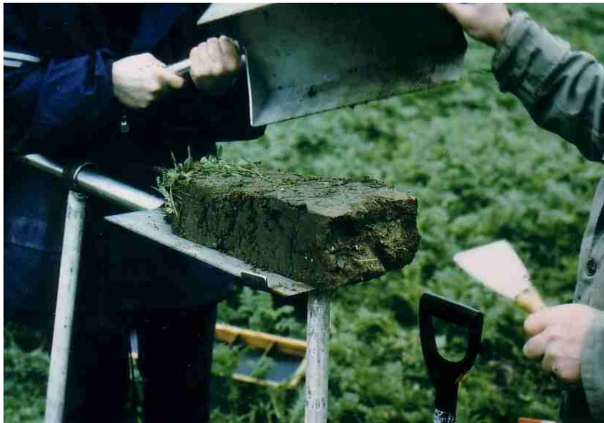
Fig. 11: Soil profile on the diagnostic stands, taking the profile spade off
